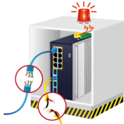
RJ45/Fiber Connection Link Down
